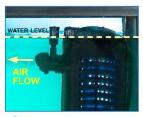
Venturi is above the water line to draw air into the water outflow.
